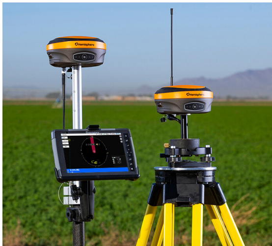
Image 2 | CNH Hemisphere (GNSS) System
